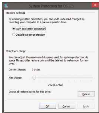
▲ System Restore takes up a lot of space – a problem for smaller SSDs
